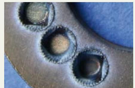
Deep engraving in a refractory Titanium alloy ablation rate 3.5 \text{mm}^3/\text{s}
