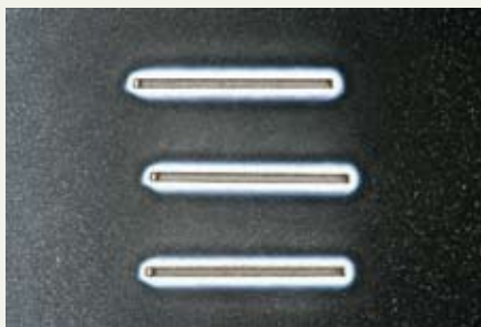
Trenching of Silicon Thickness: 725 \mu\text{m} , width: 600 \mu\text{m} , cycle time: \sim 0.3 \text{ mm}^3/\text{s}
