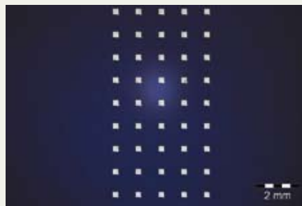
Drilling of Solar Silicon Slides Thickness: 250 \mu\text{m} , diameter: 300 \mu\text{m} , cycle time: 36 ms/hole
