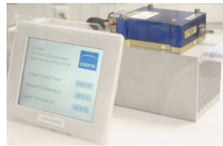
FIGURE 8: The fiber-coupled module JOLD-100-CPXF-2P A based on CN type of diode lasers delivers 100 W from a 0.4 mm fiber with a total wall plug efficiency of 42 %.
